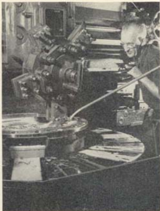
Vertical boring mill turning a turret ring for a tank.
