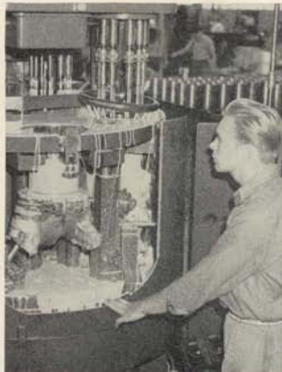
Five-position drill boring bolt holes in cylinder flange.
