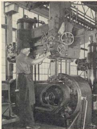
Radial drill machining a part for a tank transmission.
