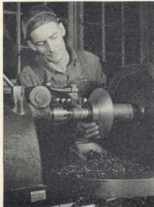
Skilled hands adjusting a gun carriage part on a lathe.
