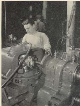
Internal grinding machine finishing plane propeller hubs.
